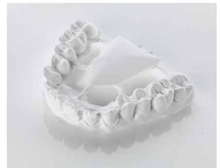
The number of connectors between the sintering block and the bridge should be at least four
